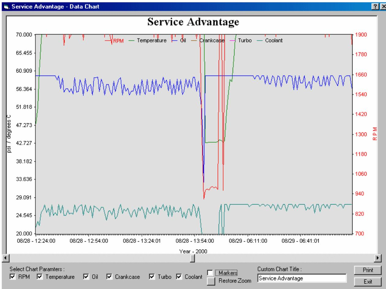
At any time you may return to the original scale by clicking the Restore Zoom button located at the bottom of the screen display.
