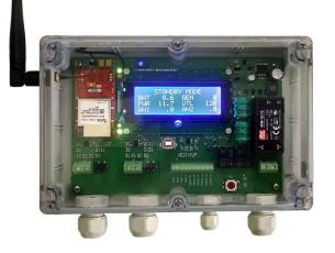
If this is the first time the monitor has been started, the radio will automatically run a provisioning sequence to activate the radio. After provisioning is successfully completed the monitor will resume standby mode.
