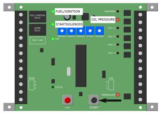
**2.** Press and hold START to manually start the generator. Allow the generator to stabilize at rated speed. Verify that the oil pressure indicator has turned off indicating that the oil pressure switch has opened.
