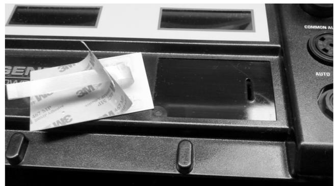
7. Insert the ribbon through the slot in the face plate. Place the keypad flush with the right edge of the recessed area and smooth out from right to left. Apply even pressure over the keypad to secure.
