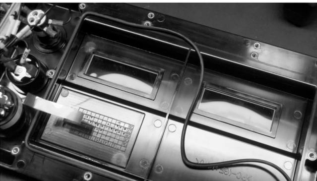
4. If the gasket is still attached to the face, gently remove the gasket from the face.
