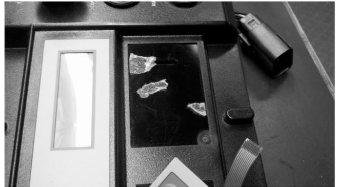
6. With the old keypad removed and the surface free of any adhesive, you are ready to install the replacement keypad. Remove the backing from the new keypad.
