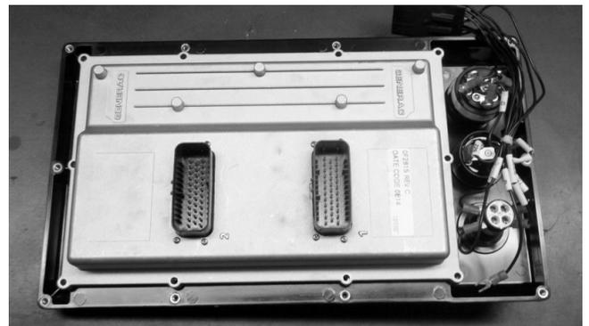
11. Insert the 10 screws that attach the face plate to the aluminum housing and secure. Remember to connect the chassis ground to the screw in the top right corner.
