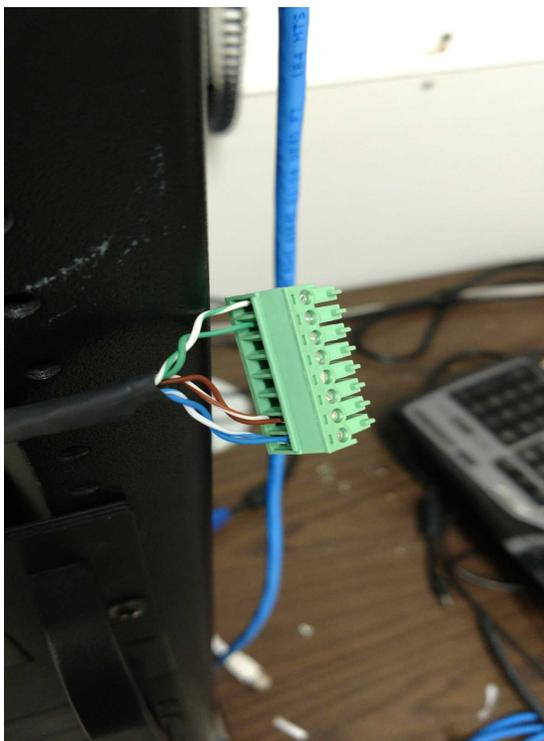
7. Now terminate the power and communication cable into the modem connector. Do not plug the connector into the modem yet. Wait until the connection has been made at the transfer switch to prevent accidentally landing a wire in the wrong position and possibly damaging the modem.
