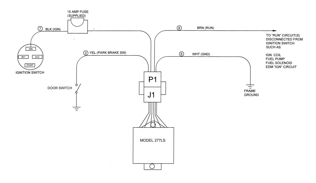
MODEL 277EC / 277LS **WIRING DIAGRAM 1** WITHOUT ACCESSORY CONTROL
