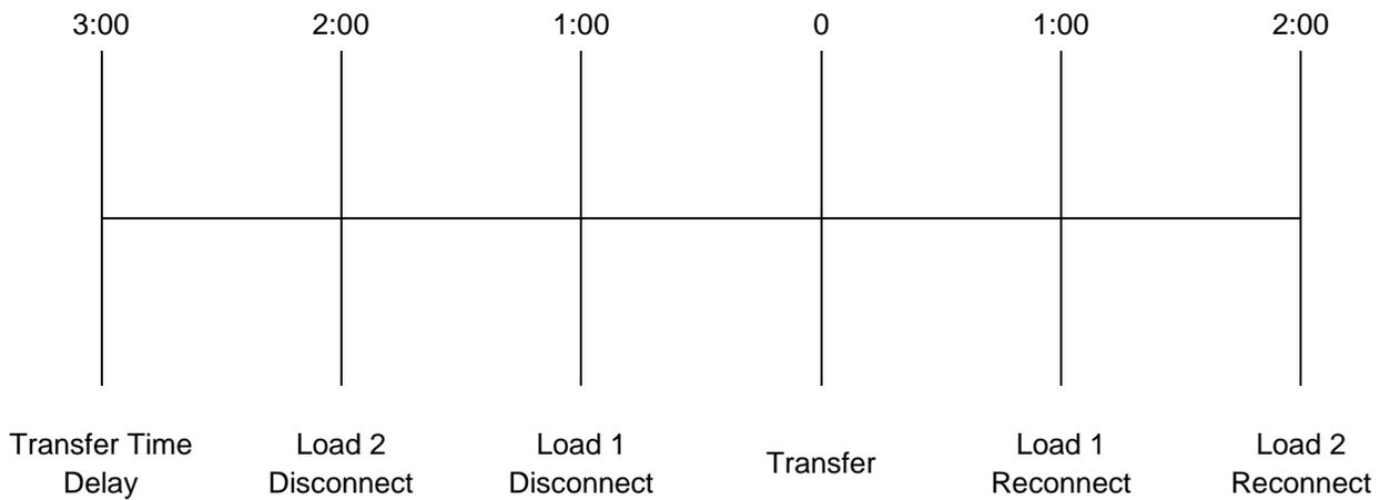
**One or more load control delays are set longer than the transfer time delay.**
