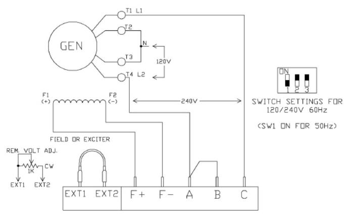
CONNECTIONS FOR 120/240V SINGLE PHASE OUTPUT FROM SINGLE PHASE GENERATOR
