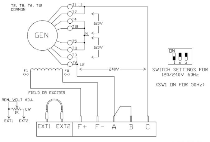
CONNECTIONS FOR 120/240V SINGLE PHASE OUTPUT FROM 3 PHASE GENERATOR (PARALLEL ZIGZAG)
