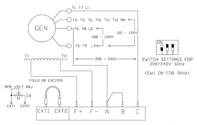
CONNECTIONS FOR 208-240V 3 PHASE DUTPUT (PARALLEL WYE)
