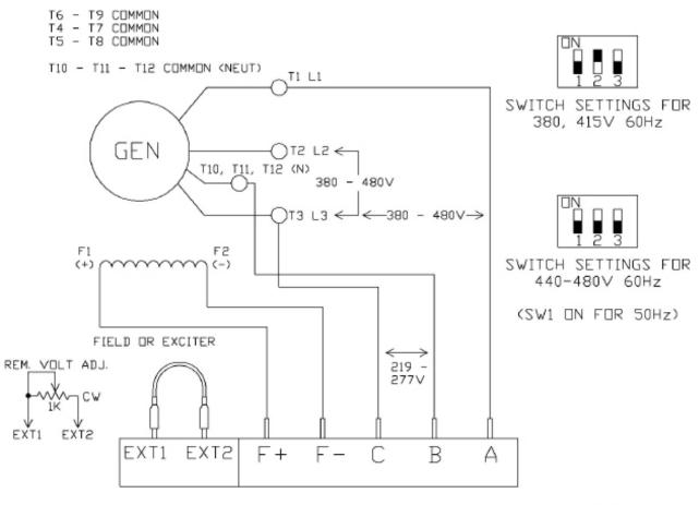
CONNECTIONS FOR 380-480V 3 PHASE DUTPUT (SERIES WYE)
