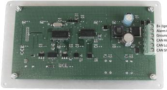
B+ (Ignition) Alarm Out (B+) Ground CAN High (Red) CAN Low (Black) CAN Shield
