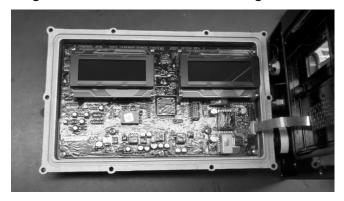
3. Gently lift up on the white connector lock to release the keypad ribbon. Remove the ribbon from the connector and separate the face from the aluminum housing.
