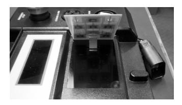
8. Place the face plate at the right side of the aluminum back, standing on edge. At this point you may want to clean the displays and the inside of the windows in the face plate. Use a soft, lint free cloth to remove dust and fingerprints. Do NOT use alcohol or other cleaners on the displays.
