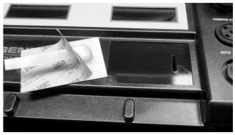
7. Insert the ribbon through the slot in the face plate. Place the keypad flush with the right edge of the recessed area and smooth out from right to left. Apply even pressure over the keypad to secure.
