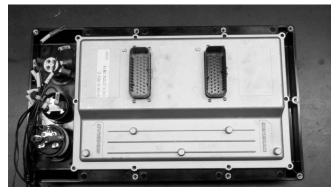
2. Turn the unit over and lift the face plate off from left to right. Stand the face plate on the right edge next to the aluminum housing.
