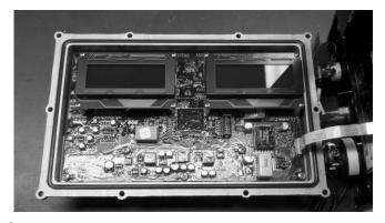
9. Insert the ribbon into the connector with the connector lock still lifted up. Be sure the ribbon is seated properly, then gently press down on the connector lock to secure the ribbon.
