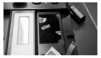
6. With the old keypad removed and the surface free of any adhesive, you are ready to install the replacement keypad. Remove the backing from the new keypad.
