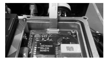
10. Now place the face plate over the aluminum housing. Be careful not to lift the face plate too far above the controller so the ribbon is not pulled from the connector. Line up the windows with the displays and be careful not to disturb the gasket on the aluminum housing. Hold the aluminum housing tight against the face plate and flip the control over.
