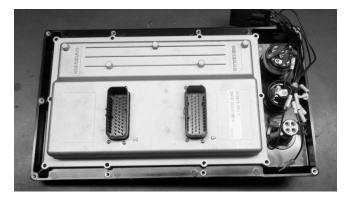
11. Insert the 10 screws that attach the face plate to the aluminum housing and secure. Remember to connect the chassis ground to the screw in the top right corner.
