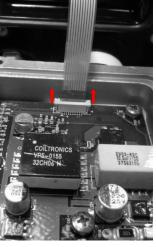
5. Remove the old keypad and use alcohol to clean up any adhesive left behind. Be sure the surface is clean and free of any oil or dirt.
