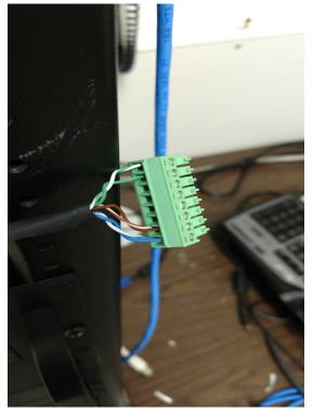
7. Now terminate the power and communication cable into the modem connector. Do not plug the connector into the modem yet. Wait until the connection has been made at the transfer switch to prevent accidentally landing a wire in the wrong position and possibly damaging the modem. 8. Next make the connections to the M328V2 observing polarity. Install the jumper for the backup battery. Secure all wiring and restore power to the transfer switch.
