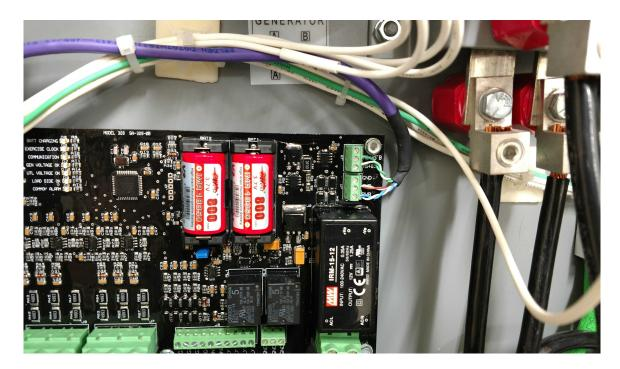
9. Check all wiring before plugging in the modem. If you are using the ethernet module, plug in the ethernet connection before applying power to the modem. Plug in the main power connector .
