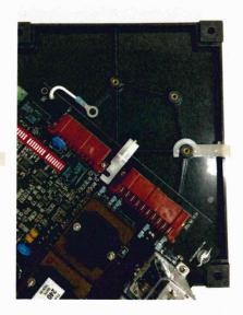
Remove the 6 mounting screws, lock washers, flat washers and plastic clip to secure cover. Install plastic clip on replacement board before installing in mounting tray.
