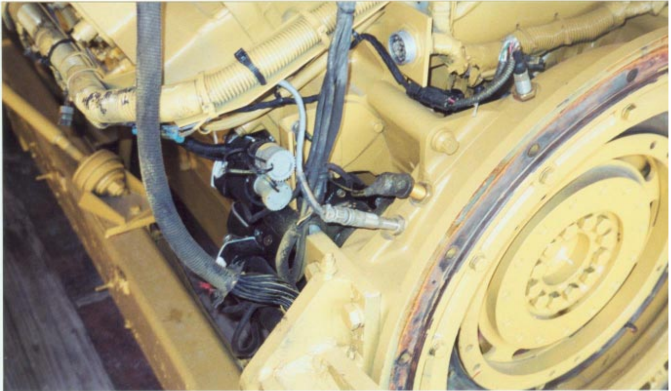
(Top) Typical mounting position of the MAG Pickup (RPM Sensor) as installed on the flywheel housing.
