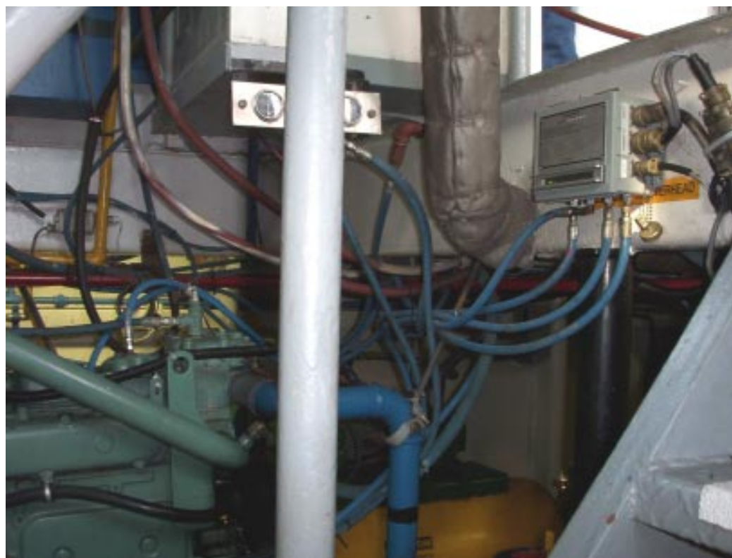
Details: Flight Systems' Model 550 Engine Saver® installed to provide protection for the Lady Jill's port Volvo 400hp Diesel.
