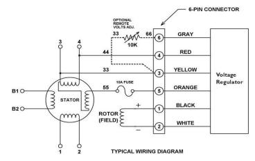
If you are replacing the regulator in a setup where power and sensing are isolated, take WIRE 66 from the generator and add it to WIRE 33 (YELLOW) wire. You can also remove the in-line diode on wire 66. It is no longer needed.
